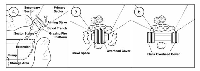
6. Build flank overhead cover if center overhead cover is impossible. Lay a support layer of logs or engineer stakes at both ends of your hole, just below ground level. Cover this with a waterproof layer of flattened boxes, a poncho, plywood or plastic sheeting, and an 8-inch protective layer of earth as a flank parapet. Dig a covered space beneath these logs.
