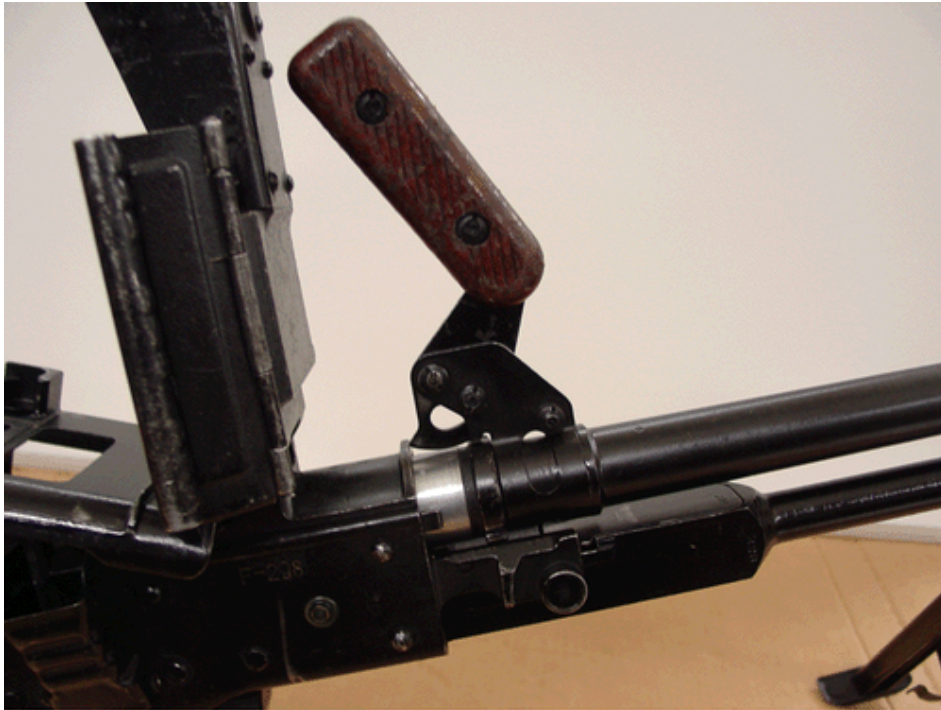
Figure 3-9. Barrel Quick-Change Handle and Barrel Pulled Forward from Barrel Receiver
