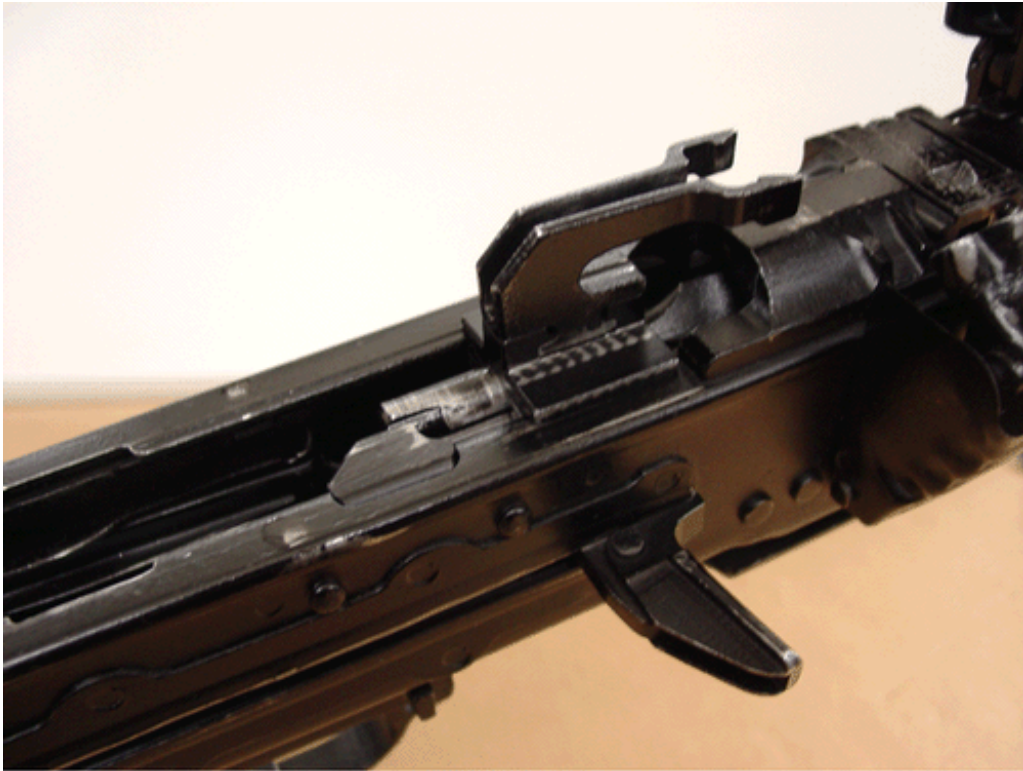
Figure 5-10. Sliding Cam and Piston in Forward Position
