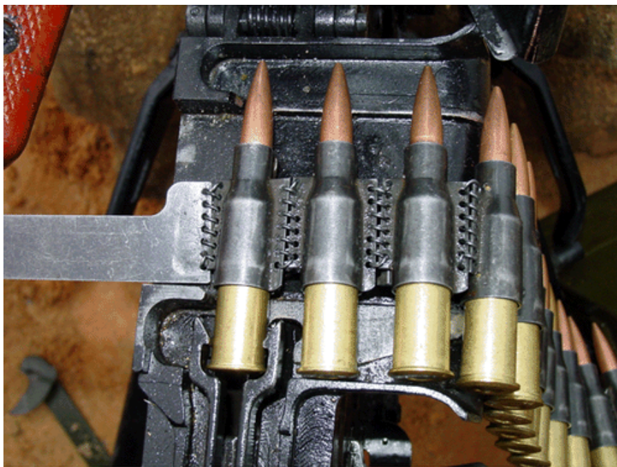
Figure 3-4. Proper Seating of Ammunition Belt in Weapon
