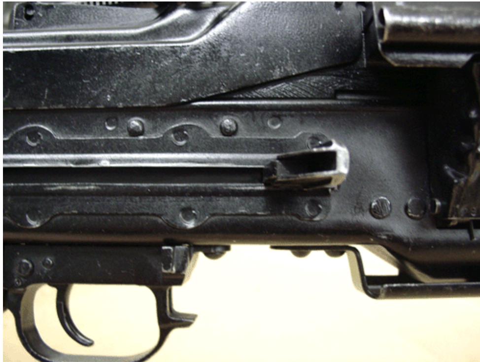
Figure 3-6. Charging Handle in Forward Position for Firing
