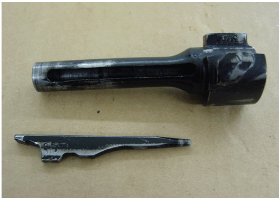
Figure 4-13. Firing Pin Pushed to Rear of Bolt
