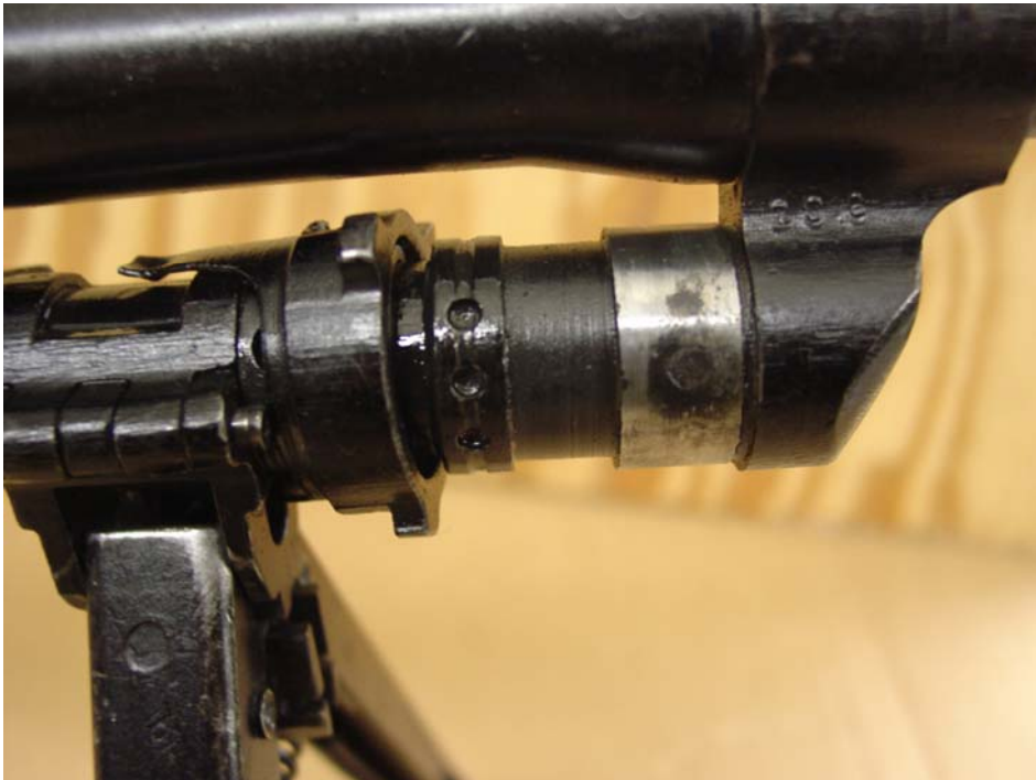
Figure 3-10. Gas Tube Seated
