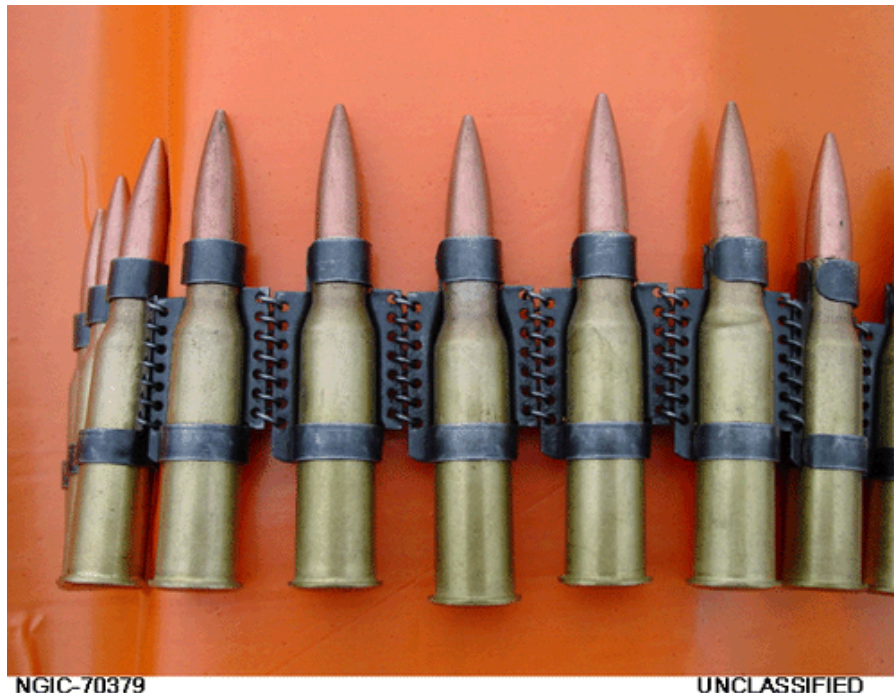
Figure 3-2. Improper Seating of Ammunition in Belt
