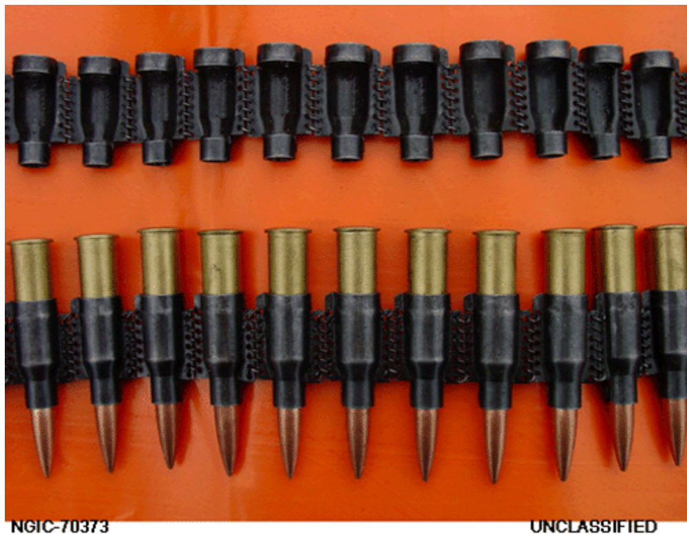
Figure 3-1. Non-Disintegrating Belt and Proper Seating of Ammunition in Belt
