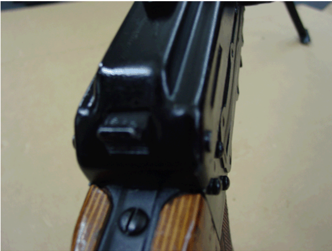
Figure 4-1. Press Feed Tray Cover Latch
