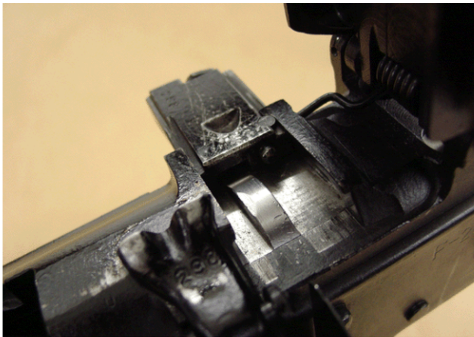
Figure 4-16. Barrel Locking Latch in Unlocked Position
