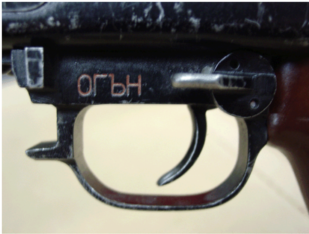
Figure 3-3. PK Selector Lever in Fire Position
