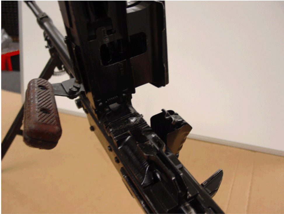
Figure 4-4. Feed Tray Raised to Full Open Position
