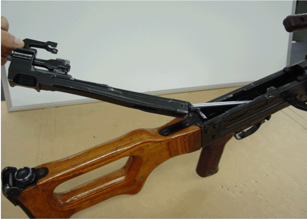
Figure 4-10. Lifting Sliding Cam and Piston from Receiver
