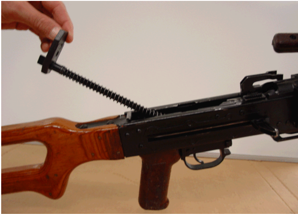
Figure 4-7. Lifting Driving Spring Rod Upward and to Rear
