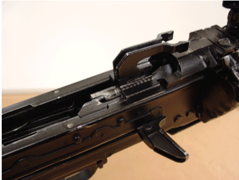
Figure 4-5. Sliding Cam and Piston in Forward Position
