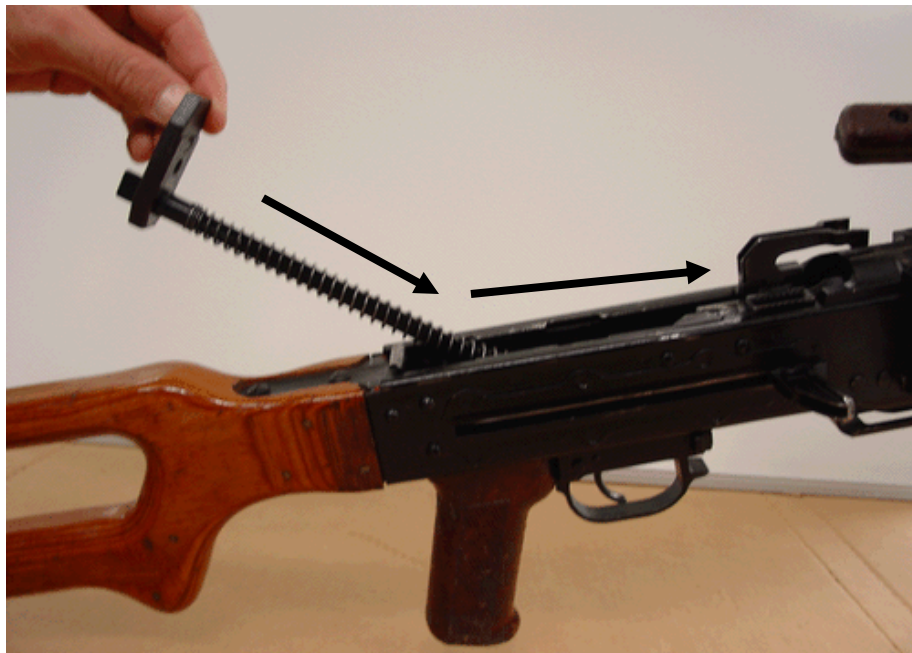
Figure 5-11. Operating Rod Assembly Aligned and Pushed Forward in Receiver Group
