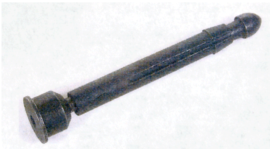
Figure 6-13. Ruptured Cartridge Extractor
