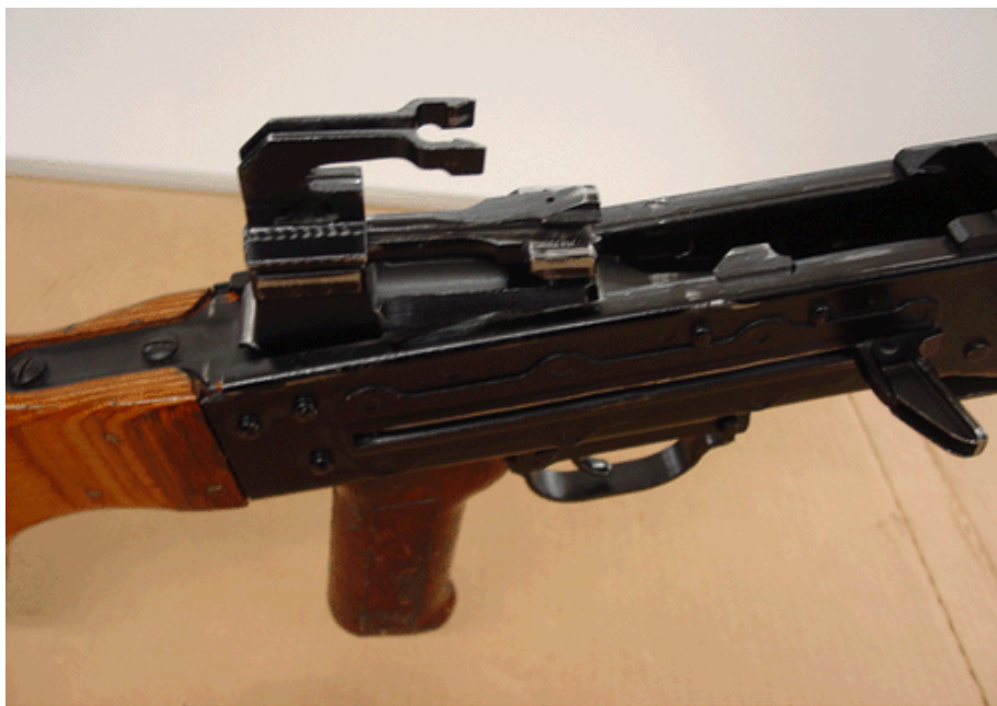
Figure 4-9. Lifting Sliding Cam from Receiver
