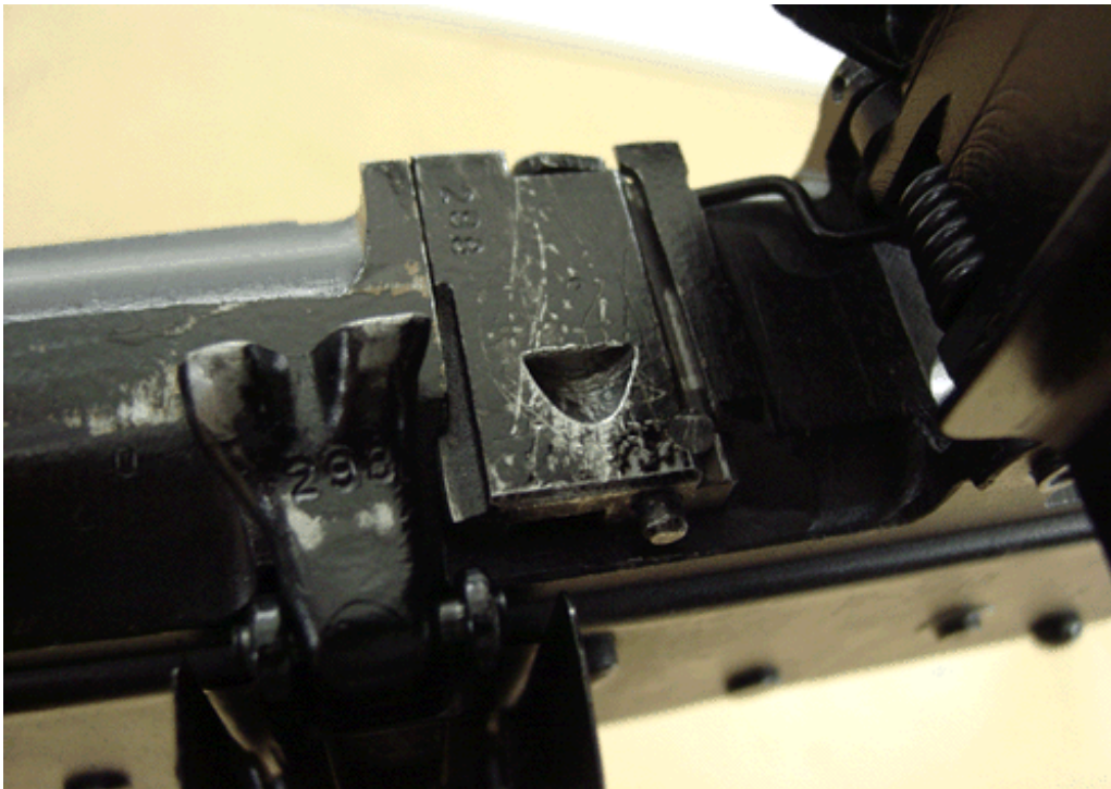
Figure 5-2. Gas Escape Chamber Aligned with Gas Regulator
