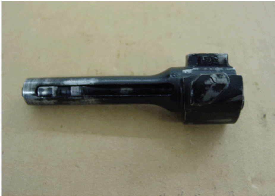
Figure 4-13. Firing Pin Pushed to Rear of Bolt
