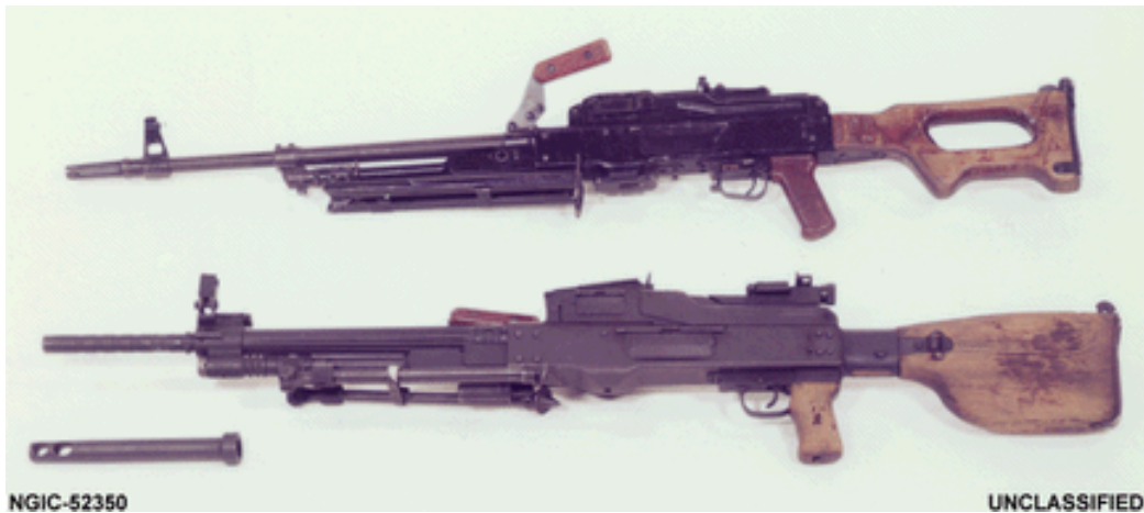
Figure 1-4. Russian PKM (Top) and North Korean Type 73 (Bottom) Machinegun
