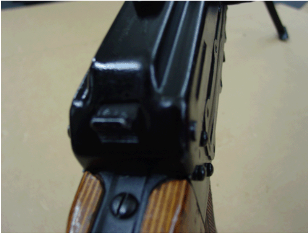
Figure 3-5. Receiver Cover Properly Closed
