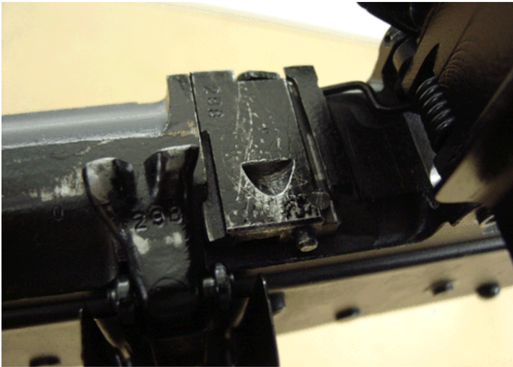
Figure 3-7. Barrel Locking Latch in Locked Position
