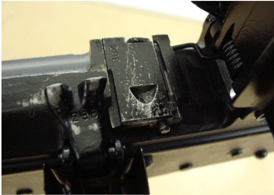
Figure 4-15. Barrel Locking Latch in Locked Position
