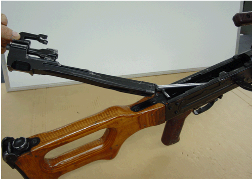
Figure 5-8. Piston Aligned into Receiver Assembly
