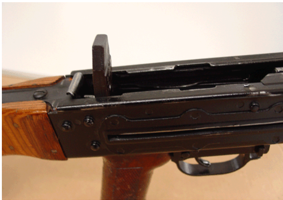
Figure 5-11. Operating Rod Assembly Aligned and Pushed Forward in Receiver Group
