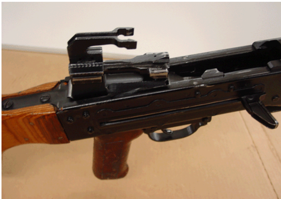
Figure 5-8. Piston Aligned into Receiver Assembly
