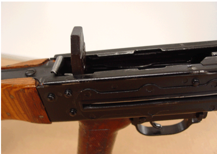
Figure 4-6. Pushing the Operating Rod Assembly Forward to Release Spring Tension
