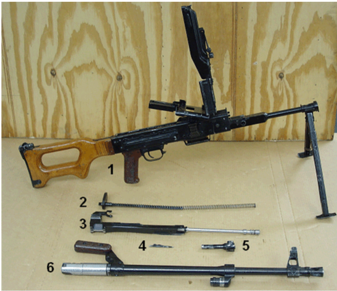
Figure 4-19. PK Machinegun Field Stripped
