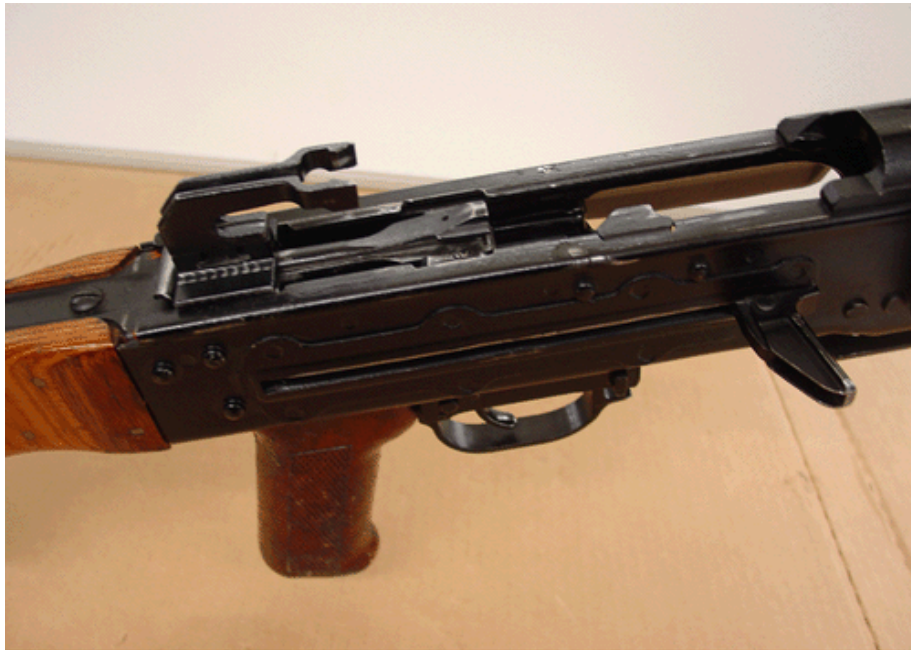
Figure 4-8. Sliding Cam Pulled to Rear of Receiver
