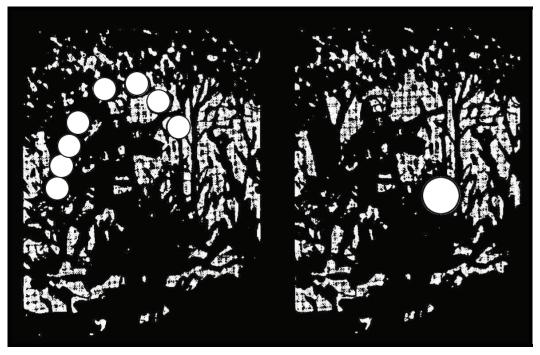
Figure J-2. Off-center viewing technique.
