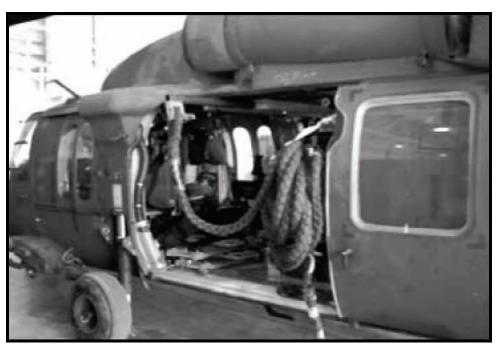
Figure 5-10. UH-60 rigged for fast roping
