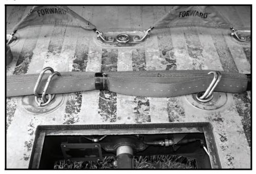
Figure 5-4. Rigging of snap links.
