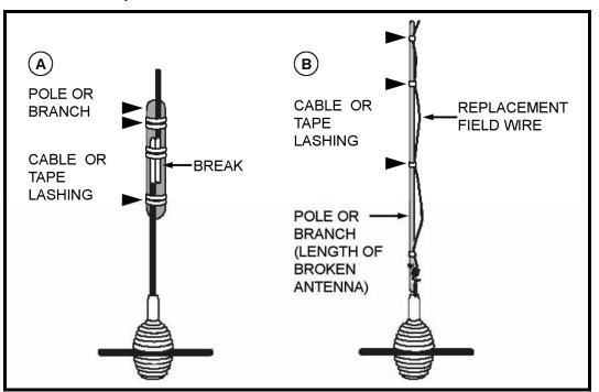
Figure 6-19. Repair procedure, whip antenna.
