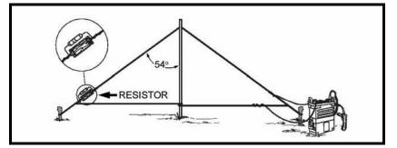
Figure 6-22. High frequency antenna, half-rhombic type.
