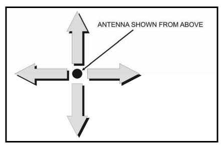
Figure 6-12. Omni-directional antenna pattern.
