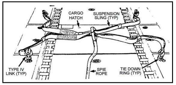
Figure 5-8. SPIES rigging procedures for CH-46 or CH-47.
