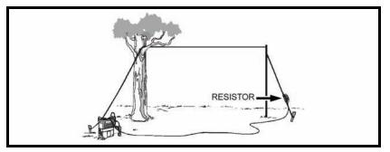
Figure 6-21. High frequency antenna, long-wire type.
