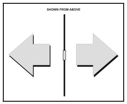
Figure 6-11. Bidirectional antenna pattern.
