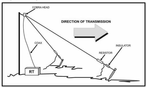
Figure 6-18. Terminated sloping "V" antenna.
