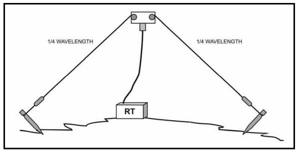
Figure 6-15. Inverted "V" antenna.
