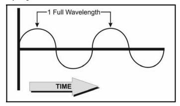
Figure 6-6. Measurement of a wavelength.
