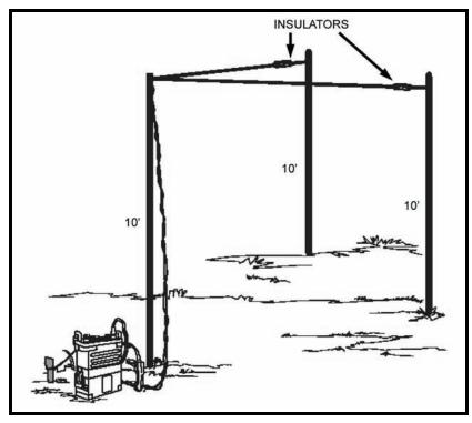
Figure 6-23. High frequency antenna, "V" type.
