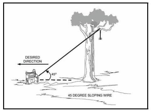
Figure 6-17. Sloping wire antenna.
