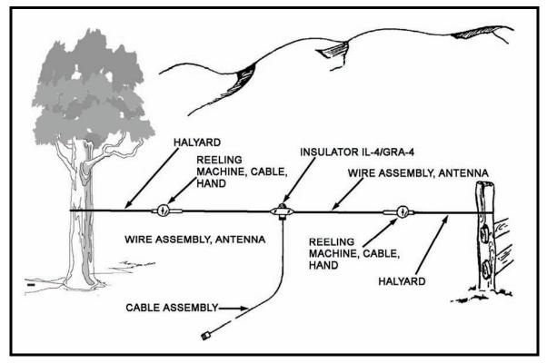
Figure 6-13. Half-wave dipole antenna.
