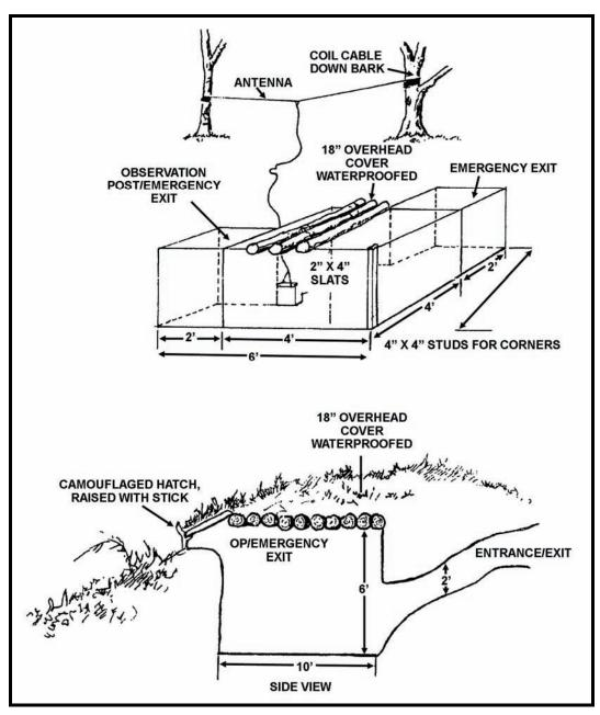
Figure G-4. Example subsurface site.
