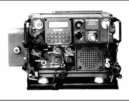
Figure 6-2. AN/PRC-150(C) in vehicular AN/VRC-104 (V)3 configuration.
