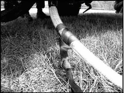
Figure 5-7. Recovery line with Prusik knot.
