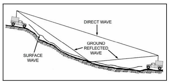
Figure 6-7. Components of ground wave.
