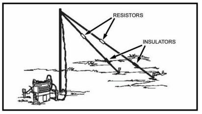
Figure 6-24. Sloping antenna, "V" type.
