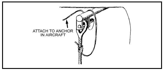
Figure 5-9. Fast-rope rigging procedures for UH-60.
