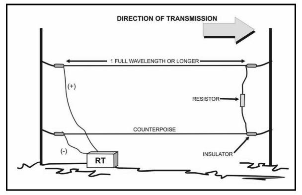
Figure 6-16. Long-wire antenna.
