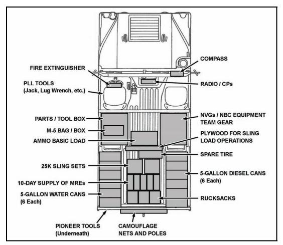
Figure 5-15. Example vehicle load configuration.
