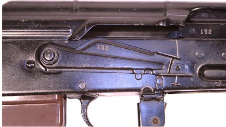
Figure 8. The Selector Lever Placed on AUTO.
