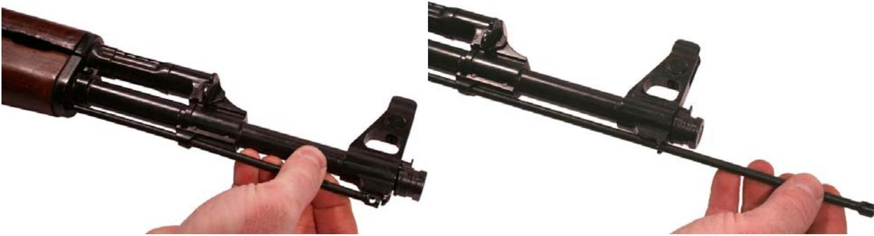
Figure 3. Removing the Cleaning Rod.
