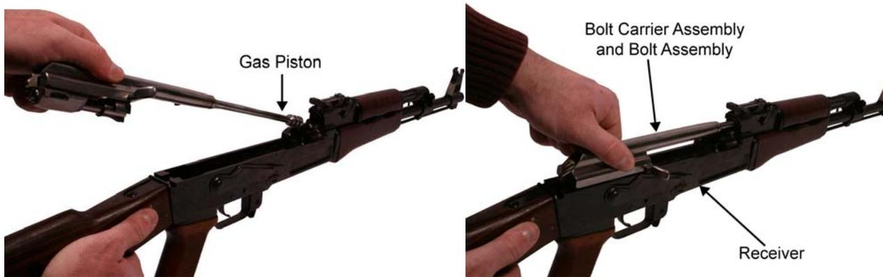
Figure 19. Inserting the Bolt Carrier Assembly and Bolt Assembly.
