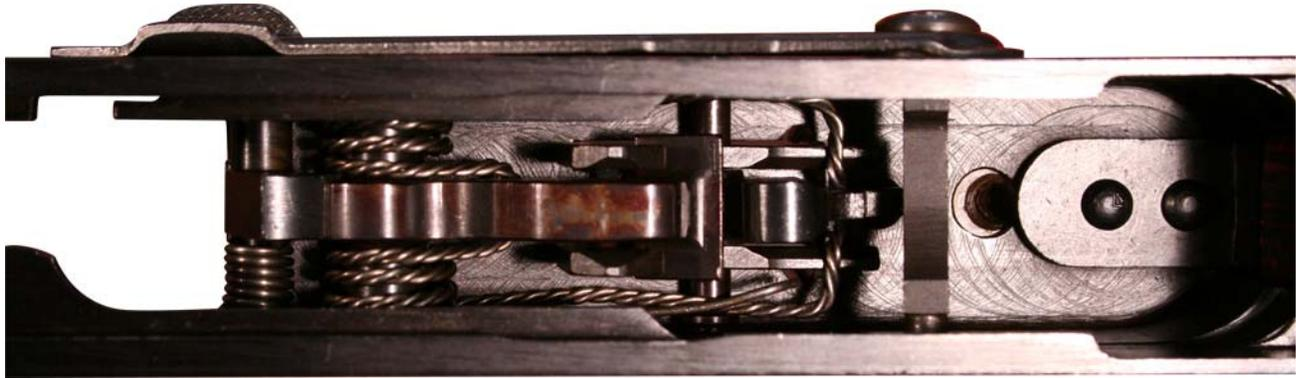
Figure 6. Moving Parts and Pins in the Receiver.
