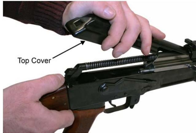
Figure 21. Installing the Top Cover.
