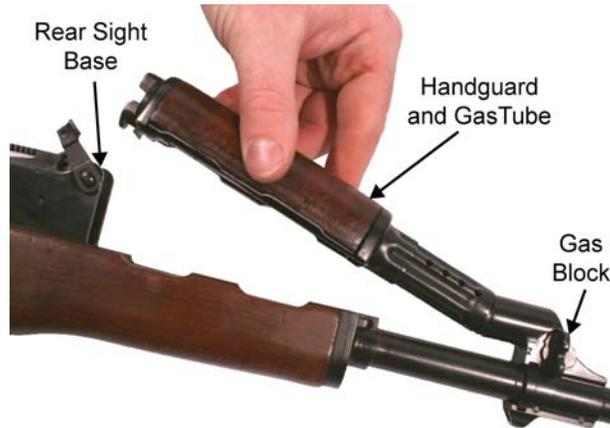
Figure 11. Removing the Gas Tube and Handguard.
