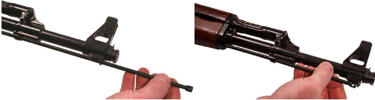
Figure 23. Installing the Cleaning Rod.
