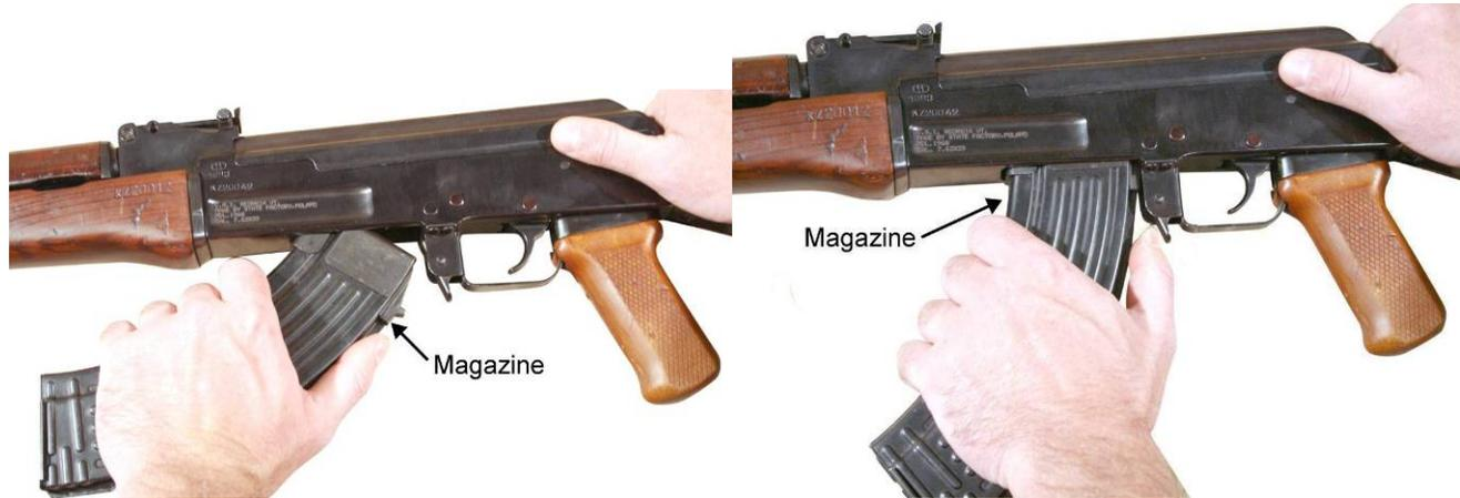
Figure 1. Inserting a Magazine.
