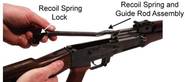
Figure 7. Lifting the Recoil Spring and Guide Rod Assembly Up and Out of the Receiver.
