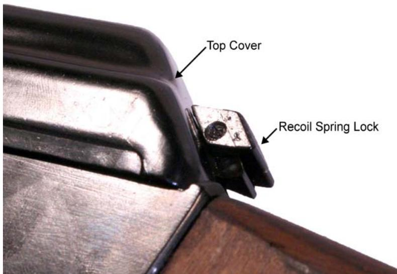
Figure 22. Two-Piece Recoil Spring Lock.
