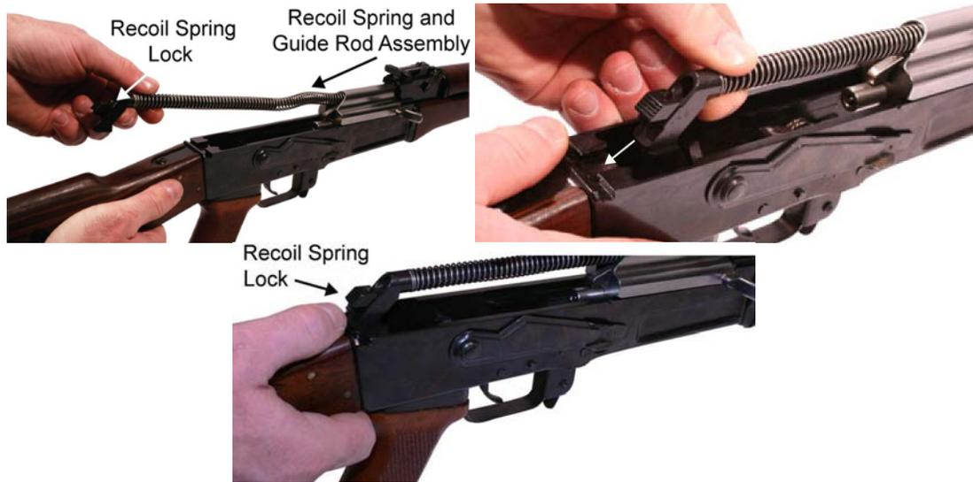
Figure 20. Installing the Recoil Spring and Guide Rod.
