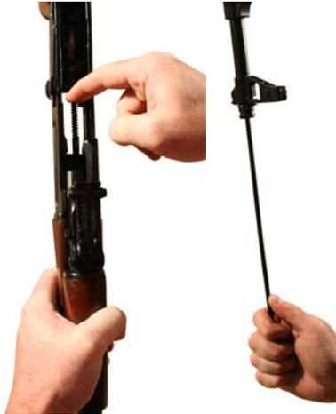
Figure 4. Running the Bore Brush through the Bore and out of the Muzzle.
