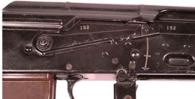
Figure 6. Selector Lever Placed on SAFE.
