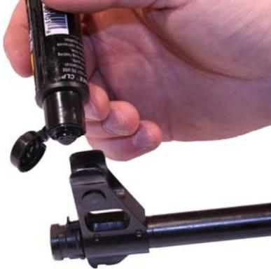
Figure 2. Lubricating the Front Sight Post.
