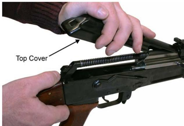
Figure 6. Lifting and Removing the Top Cover.
