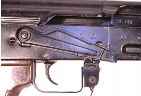
Figure 7. The Selector Lever Placed on SEMI.
