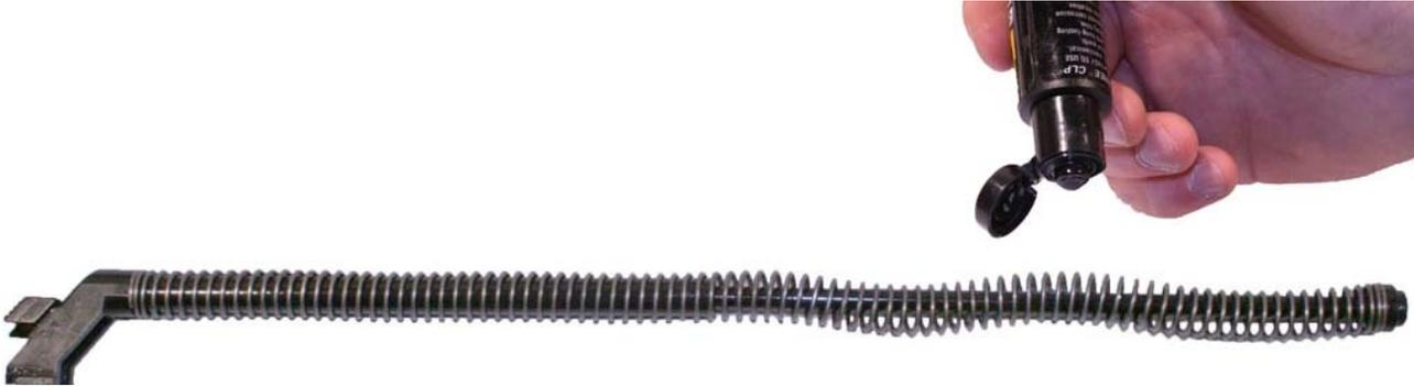
Figure 5. Lubricating the Recoil Spring and Guide Rod Assembly.
