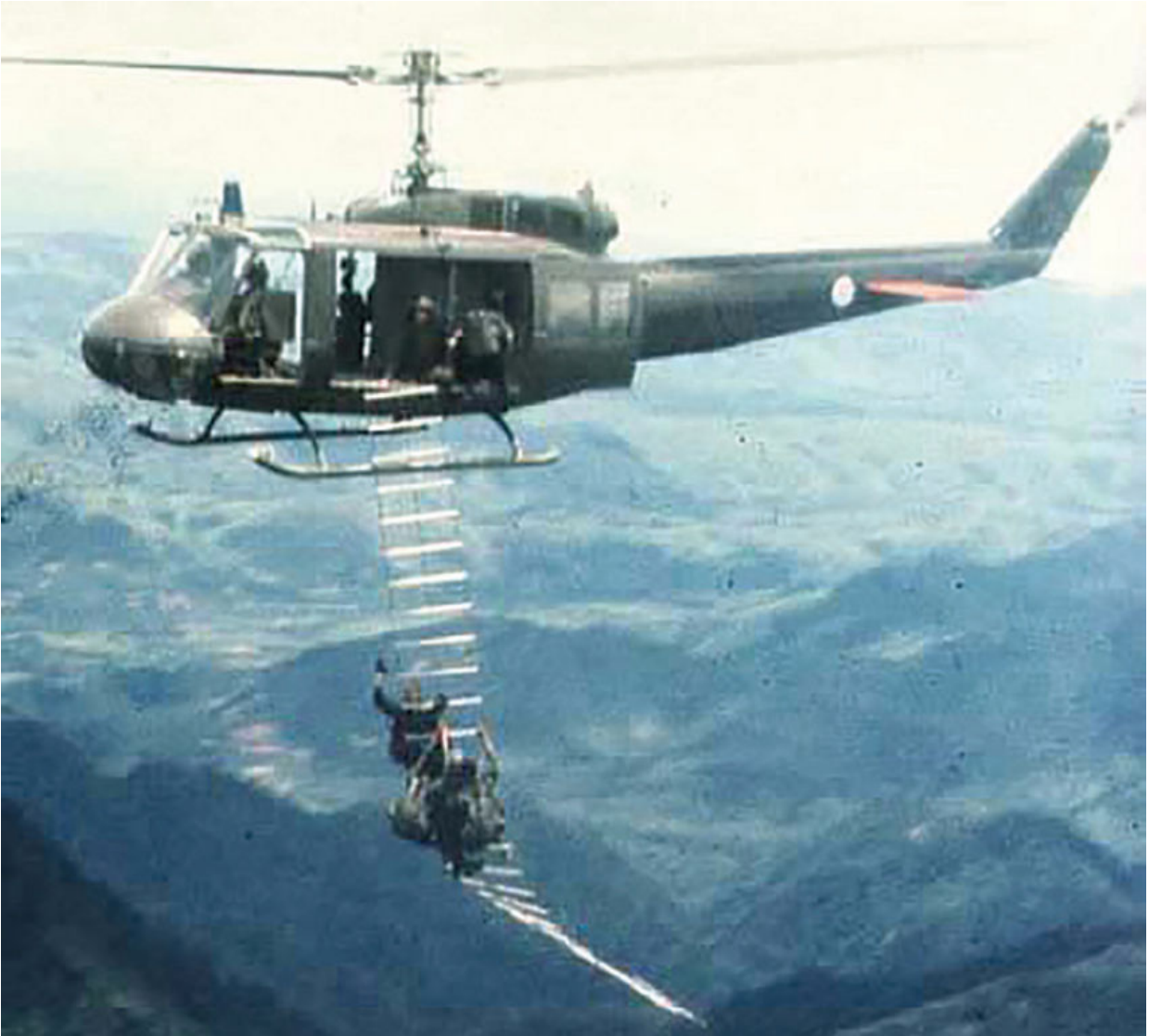
Figure 69. A ladder extraction at altitude. SOG Team Members may either ascend to the helicopter cargo bay, or may secure themselves and their equipment to the ladder with Karabiners.
