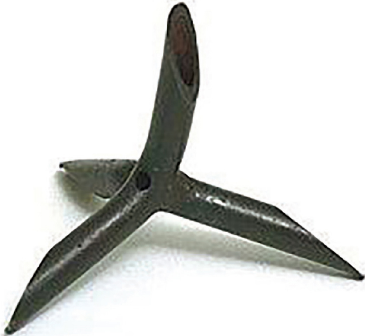
Figure 62. OSS Caltrop. Hollow spikes allow air to bleed out even if caltrop remains embedded in the tire. ( CIA Artifact - Public Domain )
