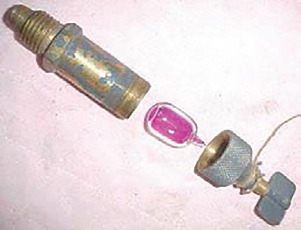
Figure 101. Limpet Mine Detonator w/ chemical delay ampoule (minus blasting cap and other kit components). ( Public Domain )
