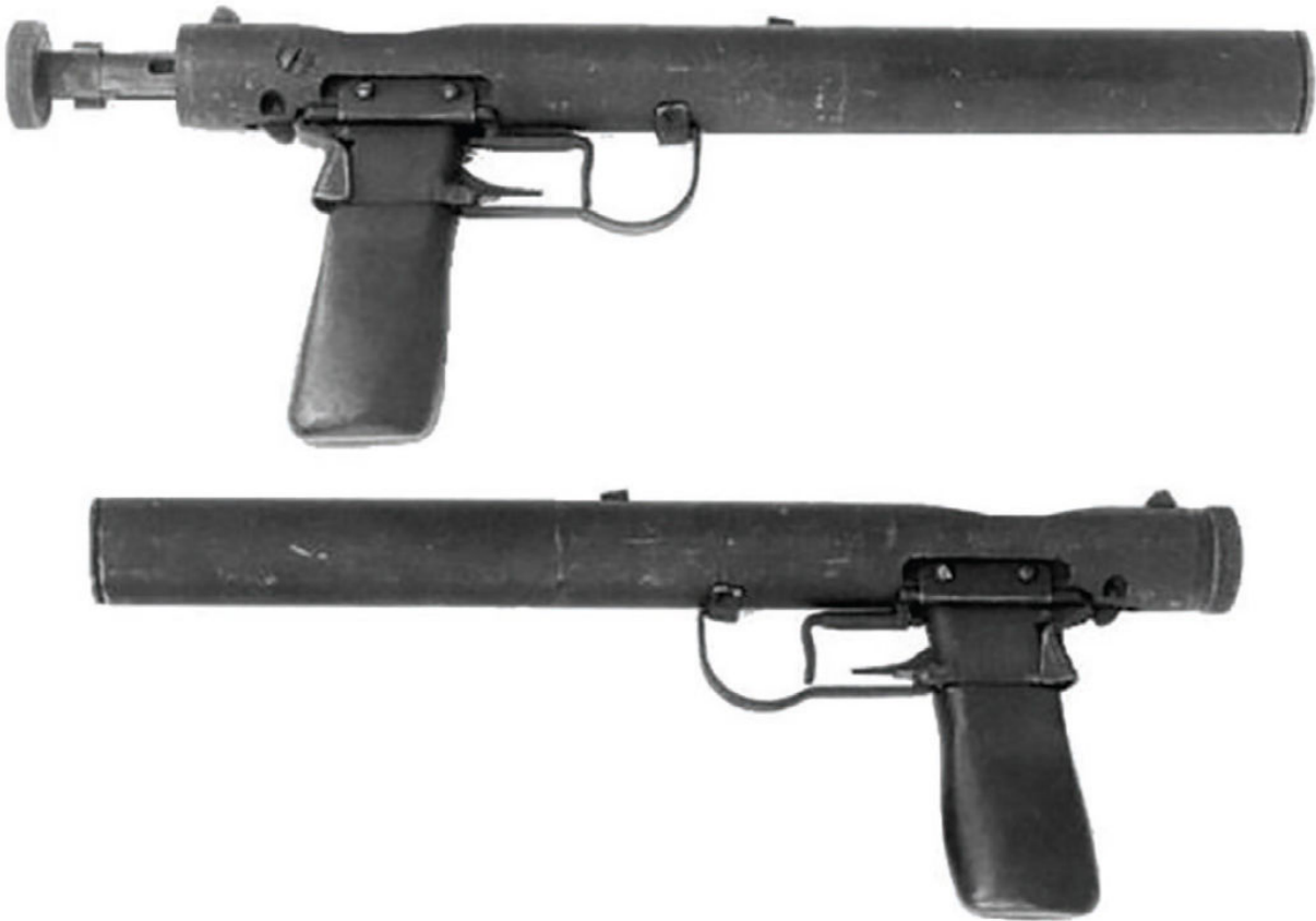
Figure 87. The Bolt Action OSS Welrod in .32 Cal. The Removable Grip is the Magazine. ( Public Domain )
