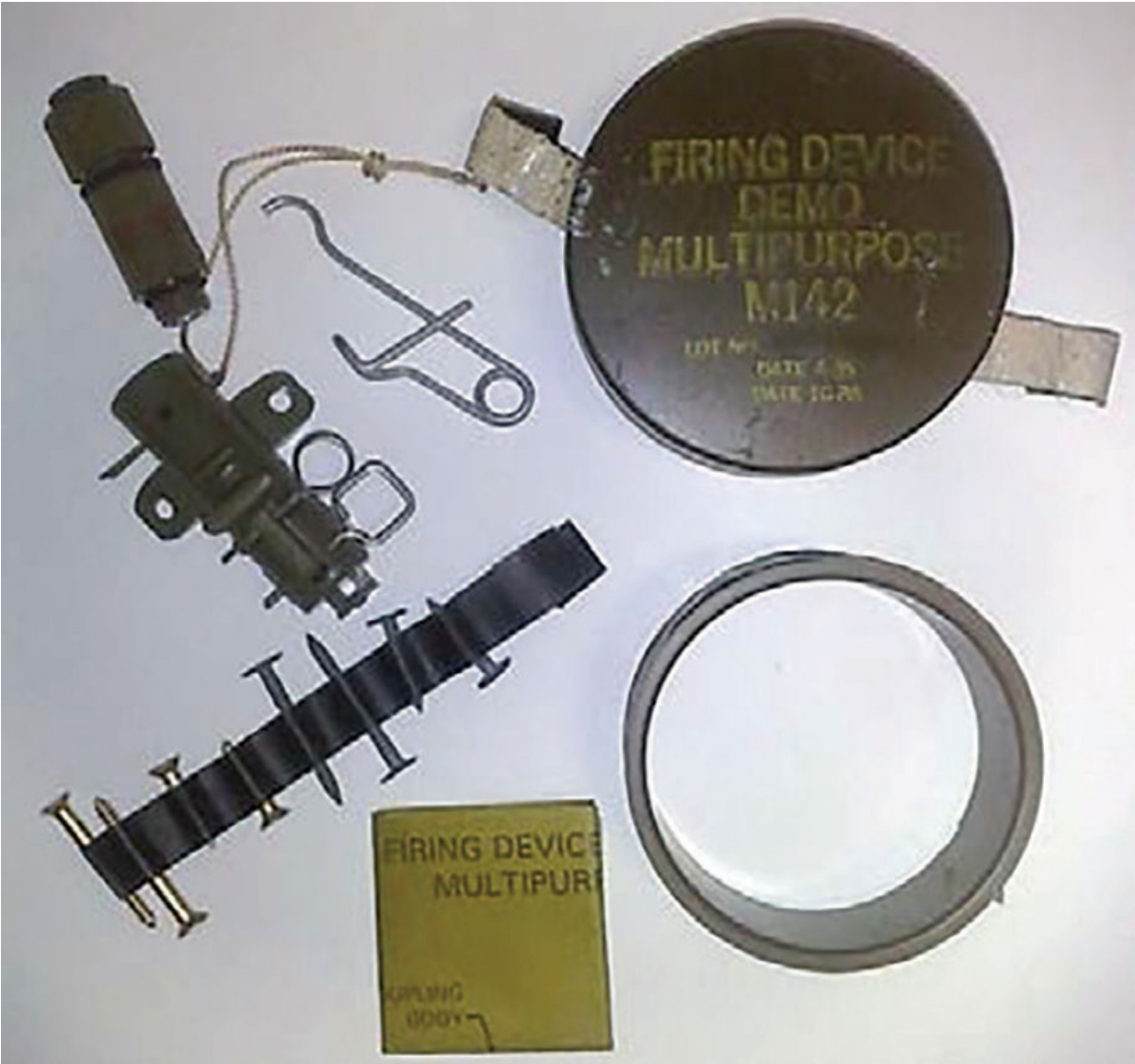
Figure 100. US M142 Multipurpose Demolition Firing Device Components. ( Public Domain )
