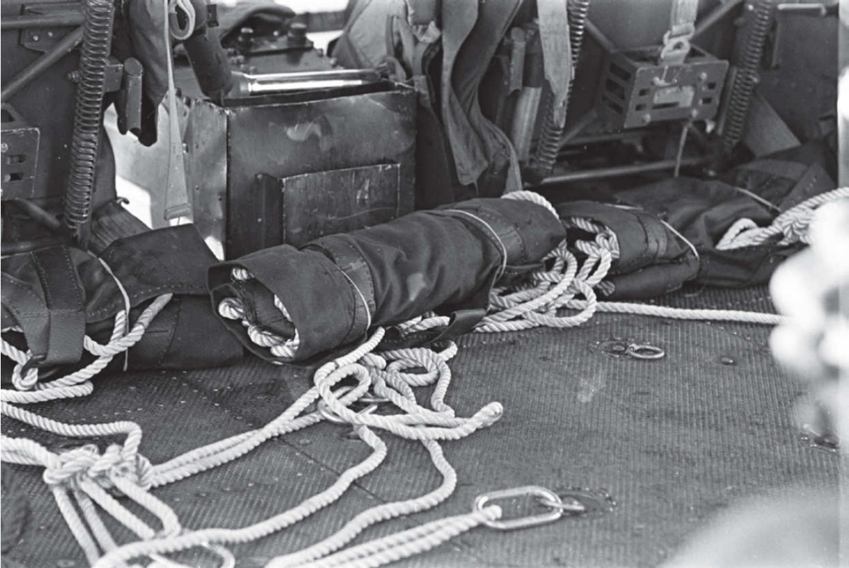
Figure 76. A “Rigger Rolled” STABO Extraction Line Contained in a Deployment Bag. ( Hardy )
