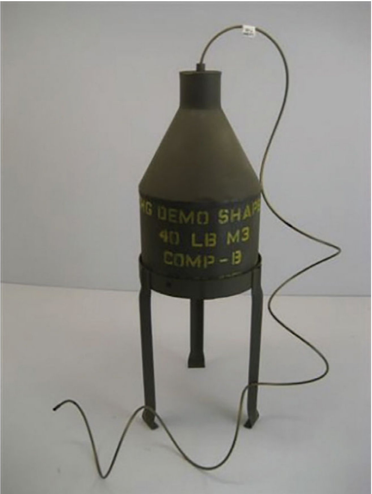
Figure 58. 40lb Shaped Charge on its stand-off legs. ( Army Photo )
